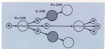
This illustration symbolizes the fast breeder nuclear reaction. A "fast neutron" hits plutonium, simultaneously releasing energy to generate electricity and a number of free neutrons(n). Some neutrons split additional plutonium atoms, sustaining the chain reaction, while others are absorbed by "fertile" uranium-238, thus being converted into new plutonium-239.
